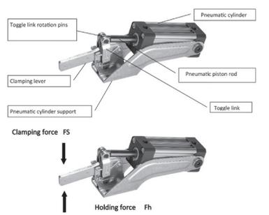
The force that a tool can express during closure is defined clamping force [FS] and the force that the tool in closed position can support without undergoing permanent deformation is called the holding force [Fh].
